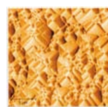
矽晶太陽能電池 Texture surface of solar cell
